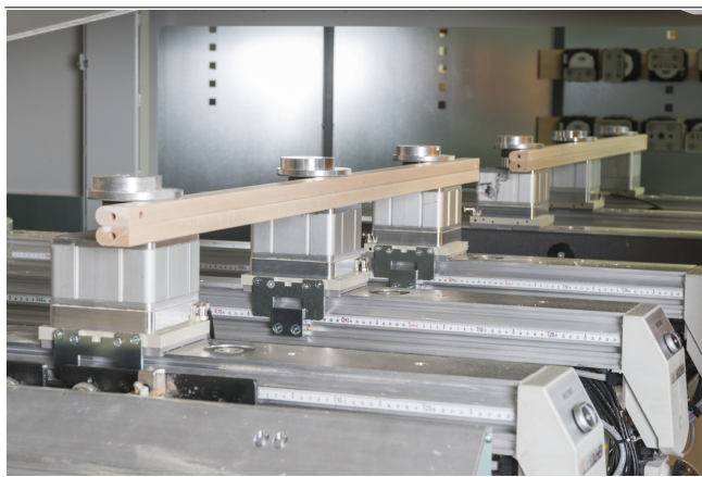
Mechanical clamps VCMC-K1 for clamping frame parts
